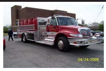
Leitchfield Fire Department in Grayson County recently took delivery on a new Pumper/Tanker. It was built by Bluegrass Fire Apparatus in Elizabethtown KY. It has a 1500 gal tank, and 1000GPM Pump all on a 2008 International Chassie, it also has a built in Foam tank.
