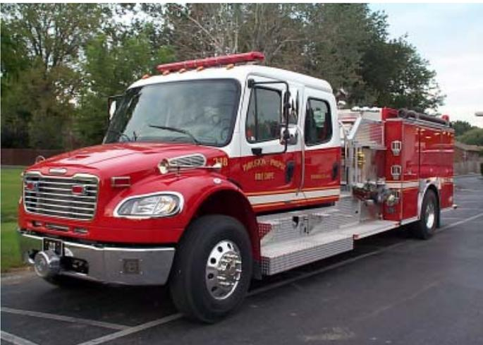
Thruston-Philpot Fire Department in Daviess County has placed a new pumper in-service (Unit 218). The 2006 Freightliner/E-One was purchased from WSF Fleet Services. The apparatus features a 5-person cab, 1250 gpm Hale pump, 1000 gallon booster tank, and much more according to Thruston-Philpot Fire Chief Bob Newman. About 75% of the funds used to purchase the truck came from dues-paying citizens in the Thruston-Philpot response area.
