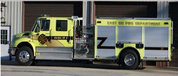
The East 60 Fire Department in Shelby Co. has taken delivery of a 2011 Toyne Legend Pumper. The unit features a 1000 gallon tank, 1250 GPM Hale Pump, Harrison Hydraulic Generator and Foam Pro 1600 class A foam system. The unit is built on an International 4400 chassis. The unit was sold by High Tech Rescue, Inc. Congratulations to Chief Steve Brookshire and the Firefighters of East 60 Kentucky.
