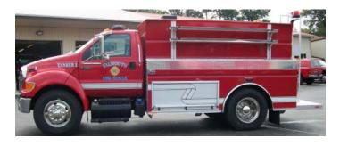
Also Delivered to Falmouth Fire Department - 2011 Wynn 500 Series Ford F-750 Tanker, with a 2000-Gallon Wetside Tanker Body, HP 200 Hale Portable Pump on Tailboard, 10" Dump Valve on rear, Dump Tank Rack on the passenger side, and much more! This apparatus was manufactured by Wynn Fire Equipment, LLC. 800-639-4966 www.wynnfire.com.
