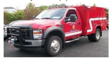
Delivered to Falmouth Fire Department - New 2010 Wynn 200 Series Ford F-550 4 x 4 Rescue, with a 9' Aluminum Body, all L.E.D. Lighting, 100-Watt Siren and Speaker, 300 Gallon Tank, 13 hp Darley Pump, and much more! This apparatus was manufactured by Wynn Fire Equipment, LLC. 800-639-4966 www.wynnfire.com.
