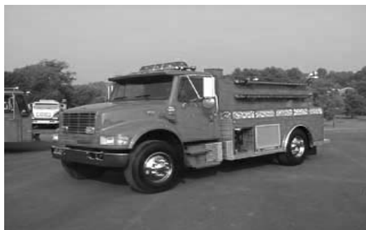
Round Mountain Fire Dept in Fayetteville Arkansas took delivery of a Wynn International Tanker. This Tanker is our standard model Tanker. It comes with a 1960 gallon tank and 400 GPM PTO Pump.
