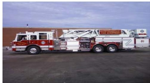
In November the City of Campbellsville placed a Velocity 95' Midmount Platform into service. It has 6 person seating capacity, a 2,000 GPM pump and a 10kw hydraulic generator. The truck was purchased with a Fire Act Grant from Pierce through Bluegrass Fire/Finley Fire Equipment Co., Inc., our local representative is John Baker.
