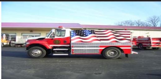
Neon Fire Dept.- Has taken delivery of a 2008 Wynn International Tanker with a 2000-Gallon Polypropylene Tank, a 14" Rear Mega Dump Valve, Portable Pump, and Swing Doors.
