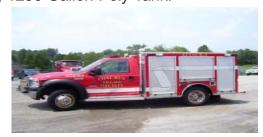
**Coal Run VFD**- 2006 Ford F-550, 4 x 4, 9' Aluminum Rescue Body with Open Top, CET C.A.F.S. Unit, 10,000# Winch and Brush Guard.
