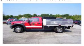
**South McCreary VFD-** 2008 Ford F-450, 4 x 4, 9' Steel Flatbed, 18 Hp CET Fire Pump, 360 Gallon Fiberglass Tank.
