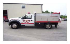
**East Knox VFD**- 2006 Ford F-450 Brush Truck, Diesel, Automatic, 4 x 4, 360-gal. Fiberglass Tank, 18 HP CET Pump, and a Scotty Foam Unit.
