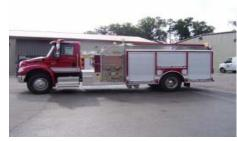
**Route 504 FD**- 2007 International, 14' Wynn Pumper Body, 1250 GPM Hale Pump, Foam Pro 1600, 1250 Gallon Poly Tank.
