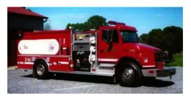
Palma-Briansburg Fire Protection District has taken delivery, of a Central States Fire Apparatus pumper-tanker, mounted on a freightliner chassis. The unit features a Hale 1250 pump with a UPF 1250 gallon tank. Two 2 1/2" direct tank fills on the rear and an air operated dump valve. The truck has a 5" front suction for drsfting.
