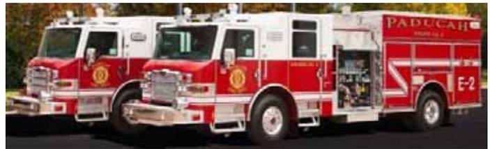
The Paducah Fire Department (Paducah, Kentucky) recently took delivery of (2) 2014 Pierce Impel Pumpers. These units feature aluminum bodies, 750 gallon poly tanks and 1500 GPM Waterous Pumps; All powered by Cummins ISL9 450 HP Engines. These units were sold by John Baker of Finley Fire Equipment Co., Inc. (800.545.3280 \* www.finleyfire.com)
