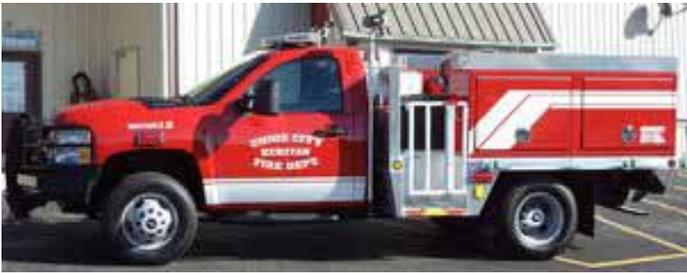
Union City Fire Dept.- Manufactured by Southeast Apparatus, LLC (888-996-6277)...A 2013 Chevrolet 3500 Brush Truck with a 9ft. aluminum flat bed, custom aluminum boxes, a Hale HPX200 Electric Start Pump with 18HP Briggs and Stratton Gas Engine, 200-Gallon UPF Polypropylene Water Tank, and much more!
