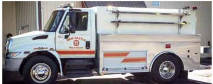
New Castle Fire Dept.- Manufactured by Southeast Apparatus, LLC (888-996-6277)...A 2007 International 4400 Wetside Tanker with an 1800-Gallon Tank, a swivel dump, Hale HPX200 Electric Start Pump, Fold Down Dump Tank Rack, L.E.D. Lighting, and much more!
