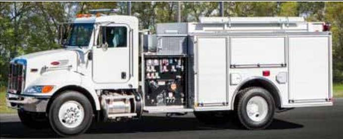
The Big Creek Fire Department (Canada, Kentucky) recently took delivery of a 2014 Pierce Commercial Pumper. This unit features an aluminum body, 1000 gallon poly tank and a 1250 GPM Waterous Pump; All powered by a Peterbilt PX-8 Engine. This unit was sold by George Owens of Finley Fire Equipment Co., Inc. (800.545.3280 \* www.finleyfire.com)
