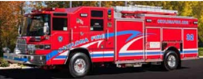
The Okolona Fire Department (Louisville, Kentucky) recently took delivery of a 2014 Pierce Quantum Pumper. This unit features an aluminum body, 750 gallon poly tank, 2000 GPM Waterous Pump, and a Husky 12 single agent foam system; All powered by a DDC DD13, 500 HP Engine. This unit was sold by John Baker of Finley Fire Equipment Co., Inc. (800.545.3280 \* www.finleyfire.com)
