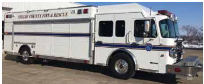
Shelby County Fire District has taken delivery of a 2014 Hackney Heavy Rescue. This unit is built on a Spartan Metro Star Chassis with an advanced crash protection system. The body features a 35KW PTO generator, dual Genesis rescue pumps, front and rear mounted extrication tools and reels, and utility air supply, and light tower. The unit was sold by High Tech Rescue, Inc.
