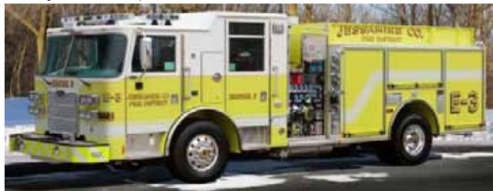
The Jessamine County Fire Department (Nicholasville, Kentucky) recently took delivery of two 2014 Pierce Arrow XT Pumpers – Engines 3 & 4. These units feature an aluminum body, 1000 gallon poly tank, a 1500 GPM Waterous Pump, and a Husky 3 single agent foam system; All powered by a DDC DD13, 500 HP Engine. These unit were sold by John Baker of Finley Fire Equipment Co., Inc. (800.545.3280 \* www.finleyfire.com)
