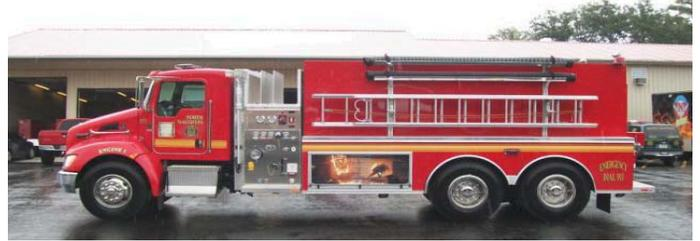
Wynn Fire Equipment, LLC recently delivered to North Magoffin VFD a 2011 Wynn Kenworth T-370 Tandem Tanker with a 750-GPM Waterous Pump, a 2700-Gallon Wetside Tank, 3000-Gallon Dump Tank, all L.E.D. Emergency Lighting, and much more!
