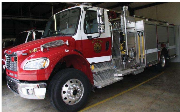
Mt. Victory- 1250 GPM-1000 gal. Tank Class A foam System. Stainless Body.
