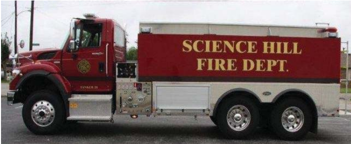
Science Hill has taken delivery on a 750 GPM-3000 gal. Tank Aluminum Body
