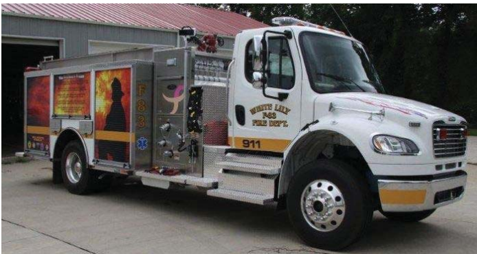
White Lilly-1250 GPM-1000 gal. Tank Class A foam System. Stainless Body.
