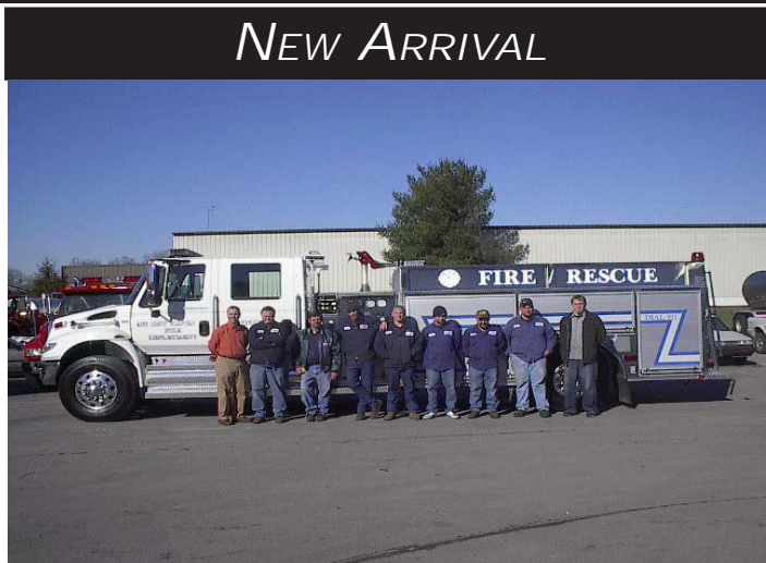
The New Haven Fire Department has taken delivery of a 2007 International 4400 Series chassis, Waterous 1250 GPM pump, with stainless steel rescue style body, 1000 gallon stainless steel tank, built by Bluegrass Fire Apparatus, Elizabethtown KY, delivered in December 2006. All items on this truck are accessible from ground level.
