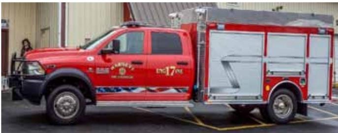
Hargett Fire & Rescue- Manufactured by Southeast Apparatus, LLC (888-996-6277)...A 2013 Dodge Ram 5500 Brush/Attack Truck with a 11ft. body, a Warn 12000 DC 12 Volt Electric Winch, Brush Guard, Transverse Slide Tray, Telescoping Scene Lights, 300-gallon tank, Scotty ATP Foam System, and much more!
