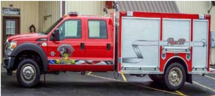
Gray Hawk Fire Dept.- Manufactured by Southeast Apparatus, LLC (888-996-6277).A 2013 Ford F-550 Rescue with Whelen L.E.D. Lighting, Push up Scene Lights, 1000# Dual Direction Slide Tray, Line-X Bed Liner, 300-gallon polypropylene tank, and much more
