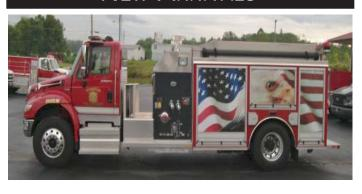
Webster Fire Department has taken delivery of a 2009 Wynn 600R Series International Pumper with a Darley 1250-GPM Pump with Top Mounted Controls, a 200 CFM Darley CAFS, a 20-Gallon Integrated Foam Tank, and a 1000-Gallon Polypropylene Tank.
