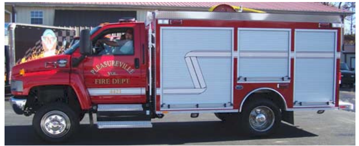
Pleasureville Fire Dept.- 2009 GMC 5500, Wynn 12' Aluminum Body, 50 CFM CET CAFS Unit, 300-gal. Polypropylene Tank, and Yamaha Generator.
