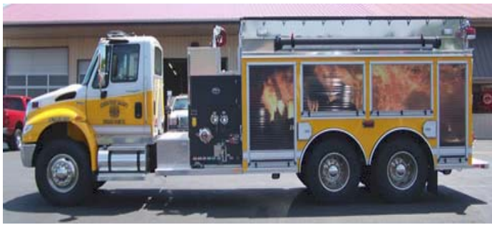
Kite-Top Most Fire Dept.- 2010 International Tandem, Wynn 1600 Series, 1250-gpm Darley Pump with a FoamPro System, 2000-gal. Polypropylene Tank with a 20-gal. Foam Cell.
