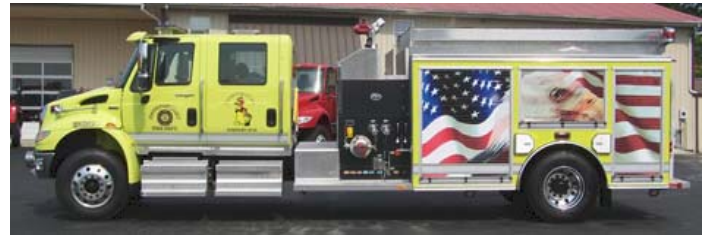
Southeast Casey Co. Fire Dept.- 2010 International Pumper, Wynn 600 Series Pumper Body, 1000-gal. Polypropylene Tank with a 20-gal. Foam Cell, 1250-gpm Darley Pump Top Mounted Controls with Foam, and miscellaneous equipment.
