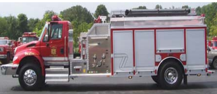
Nancy Fire Dept.- 2010 International Pumper, 1500-gpm Hale Pump with a FoamPro 1600 System, 1500-gal. Polypropylene Tank, Dual Arm Hydraulic Ladder Rack.
