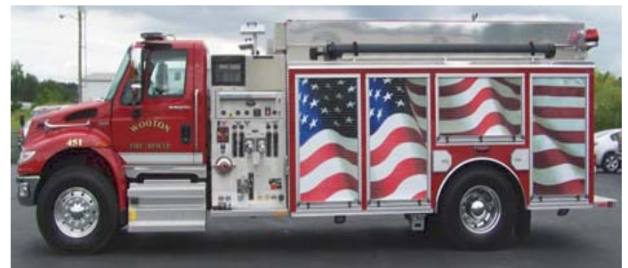
Wooton Fire Dept.- 2010 International Pumper/Tanker, Wynn 600 Series, 1250-gpm Darley Midship Pump (Side Mount) with Foam, 2000-gal. Polypropylene Tank.
