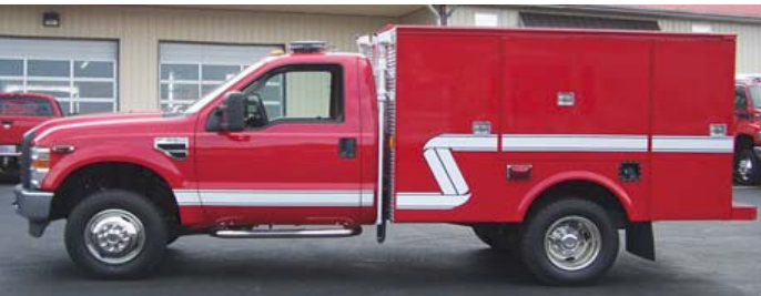
May's Lick Fire Dept.- 2009 Ford F-350 4 x 4 Rescue, 9' Rescue Body, 60-gal. CAFS Unit, Telescoping Lights.
