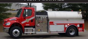
Valley Creek V.F.D. recently took delivery from Bluegrass Fire Apparatus a Freightliner M2, 330hp - Single Axle - Darley 750 PTO, - 2,000 Gallon Stainless Steel Elliptical Tank, - 10" Newton Dumps on the driver, passenger sides and rear, LED Light Package.
