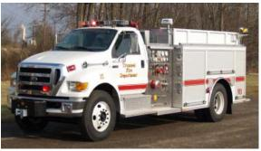
The above truck was delivered to the Trammel V.F.D. It is a Ford F-750, 260hp - Single Axle - Darley 750 PTO, 1,000 Gallon Stainless Steel Ttank, - High Sides both sides, Apollo Deck Gun, LED Light Package.
