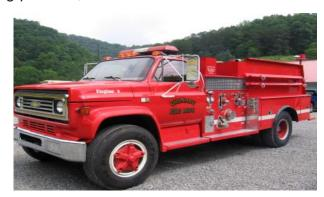
The second truck is a 1982 Chevrolet Commercial Pumper with a Detroit Diesel Allison Fuel Pincher Engine, 10 speed split manual transmission, hydraulic brakes, American LaFrance 1000 GPM 2 stage midship pump with side pump panel, Hale priming pump, 1000 gallon aluminum tank (new in 2001), discharges 2 - 2 1/2" and suction 1-2 1/2" & 1 - 6" & 2 - 1 1 1/2" crosslays. Selling price \$12,500. For more information on either truck call the Gulnare VFD Chief Philip Smith, cell (606) 794-1700.
