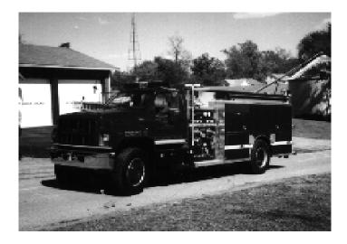
The City of North Middletown, (Bourbon County) has placed in service a 2001 Central States Fire Apparatus pumping engine. Under the direction of Chief Jeff McFarland, the response area includes the City and surrounding County areas. The unit, mounted on a GMC 7500 series chassis, has a 300 HP Caterpillar engine and Allison automatic transmission. Design features allow it to act as an "attack" apparatus or a tanker.
