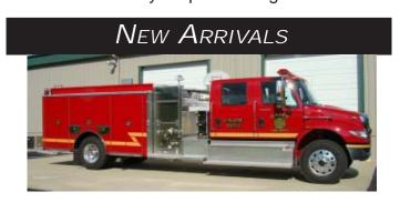
The fire truck at the bottom of the column to the left was delivered by High Tech Rescue, Shelbyville Ky. to the Waddy Fire Department in Shelby County it is a 2009 Toyne on a International Chassis with 1000 gal. Poly tank. The unit also features a 1250 GPM Hale Pump, and a Honda EM5000 generator set.
