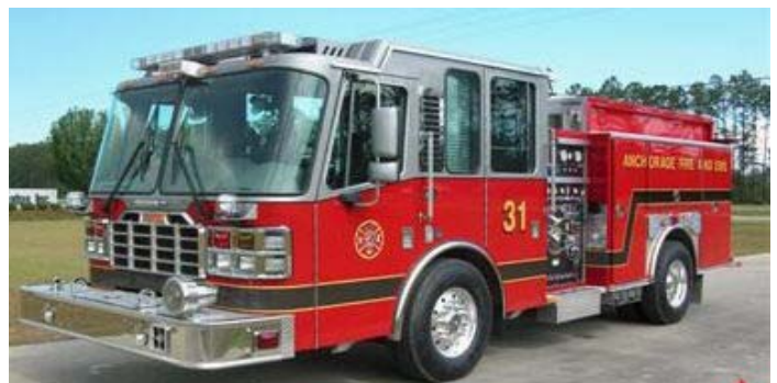
Chief Walter Lage and Anchorage Fire Dept recently took delivery of a Ferrara Igniter Custom Chassis. The Body type is Heavy Duty Extruded Aluminum with a Detroit 435 HP engine and an Allison 4000 EVS Automatic Transmission. The pump is a Waterous CSU, Single Stage, 1500 GPM connected to a 700 gallon tank.
