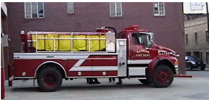
Delivered to Harlan Ky. Fire Department a Firovac 2000 gallon vacuum on a Sterling Acterra chassis with an ISC 315 engine, portable pump, portable tank with swing down bracket. It self loads from any water source at 1000-1500 GPM. “I originally saw a Firovac demonstrated at the State Fire School in Lexington, Kentucky several years ago, then again at FDIC in Indianapolis, Indiana. I was impressed with the speed and ease of loading and unloading water. After watching another demonstration here in Harlan, of water being obtained 40’ down a steep embankment and again out of a very shallow area of out river, I was sold. We took delivery of a 2000 gallon Firovac unit in September of 2006. We have never regretted the decision: it is truly a water moving machine.” Chief Linette M. Hutchison.
