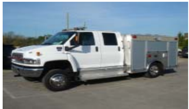
Bluegrass Fire Apparatus delivered to the Hanson Volunteer Fire Department a Stainless Steel Rescue Body on a GMC 5500 4-door chassis. The Hanson Volunteer Fire Department, located in Hanson, is about 35 miles south of Henderson Kentucky.
