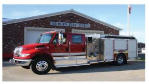
The City of Burgin has taken delivery of a 2013 Toyne pumper. This unit features a Stainless Steel Body, 1000 Gallon Poly Tank built on an International 4400 Crew cab Chassis. The unit was sold by High Tech Rescue Inc.
