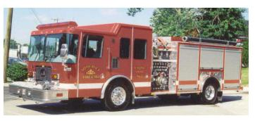
Somerset Fire / EMS took delivery of this new 2003 Ferrara custom pumper. This pumper is a 6-man cab on a HME chassis with 1250 Hale pump, 1000 poly tank, and 20-gallon foam tank. It is housed at Station 2, which services area outside the City of Somerset and as backup to the City of Somerset. It was purchased by funds from the Pulaski Fire Commission and the City of Somerset.
