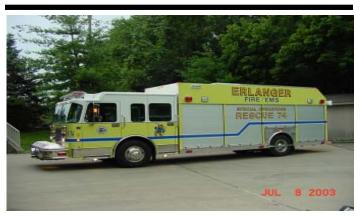
Erlanger Fire/EMS Department has taken delivery of a 2003 Rescue Truck. Summit Fire Apparatus of Edgewood, Kentucky built this apparatus. This new unit replaces a similar truck that was destroyed in a collision with a CXS freight train. This unit is built on a Spartan Advantage Chassis. This unit will respond to emergency calls involving Auto Extrication, Haz-mat, High Angle Rope Rescue, Trench and Confined Space Rescue and Structure Fires.
