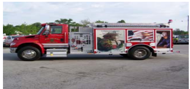
Kite-Top Most V.F.D.- 2008 International Wynn 600 Series Pumper, 1250-GPM Darley Pump with FoamPro, 1000-Gallon Polypropylene Tank
