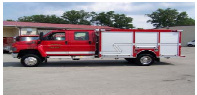
Lewisburg V.F.D.- 2008 GMC 4 x 4 Wynn 300 Series Rescue, 12' Rescue Body, 30-Gallon Stored Energy CAFS Unit.
