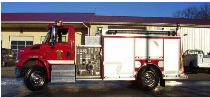
Evona- 2006 International Pumper, Waterous Pump Module with Foam Package, and a 1250-gallon Poly Tank.
