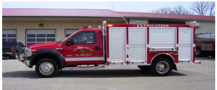
South McCreary- 2006 Ford F-550 Rescue, 6.0 Litre Diesel Engine, 11 Custom Built Aluminum Rescue Body.
