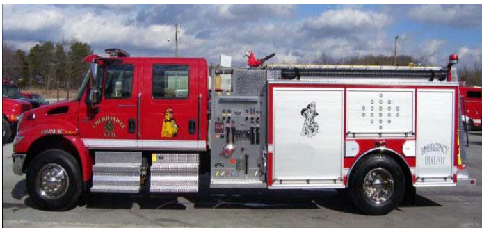
Cherryville FD- 2007 International Pumper, DT570 Engine, 1250-gpm Darley Side Mount Pump, and 1250-gallon Poly Tank.
