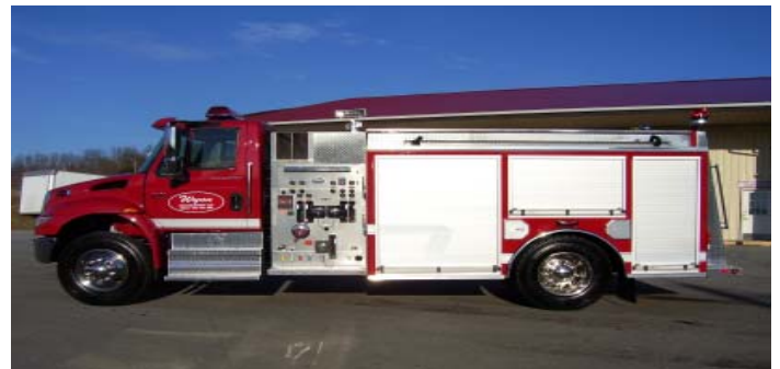
Hatfield- 2007 International Pumper, DT570 Engine, 1250-gpm Darley Pump, and a 1000-gallon Poly Tank.
