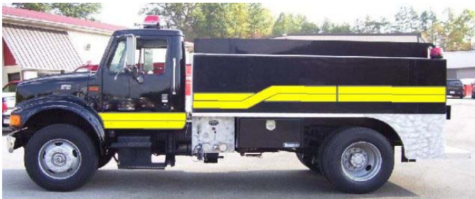
North Pendleton- 1996 International Tanker, DT466 Engine, 400-gpm Gorman Rupp Pump, and 2000-gallon Poly Tank.
