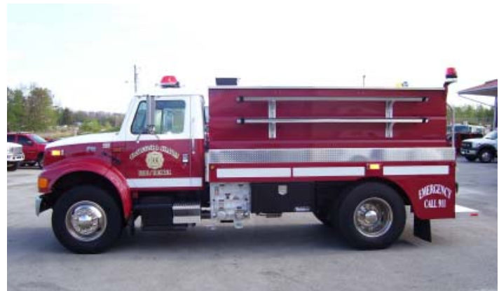
Grapevine/Chavies- 1995 International Tanker, DT466 Engine, 400-gpm Gorman Rupp Pump, and an 1800-gallon Poly Tank.
