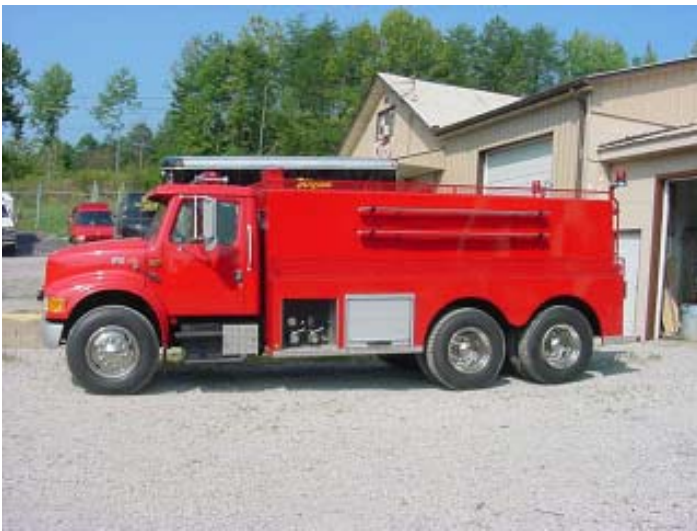
1996 International Tanker built by Wynn Fire Equipment for Buck Head Fire Dept. in NC. 2700 gal. tank 400 gpm PTO pump.
